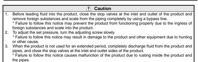
5. The set pressure may be affected by ambient temperature (external temperature) and fluid temperature. Install pipes so that the product may not be exposed to direct sunlight.
