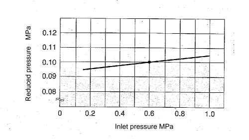
This chart shows variation in the reduced pressure when the inlet pressure of 0.60 MPa is changed between 0.15 MPa and 1.0 MPa after the reduced pressure is set at 0.10 MPa.
