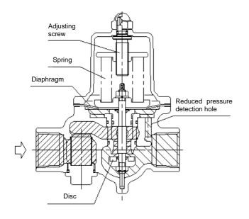
The spring is compressed by the adjusting screw, the diaphragm is pushed down, and thereby the disc directly connected to it is opened.
