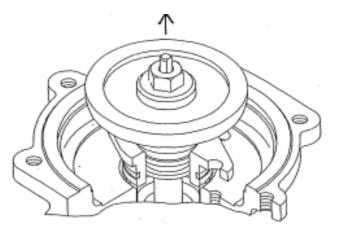
Nominal size 65A to 100A: Screw the bolt into the valve seat [3], and pull it up.
