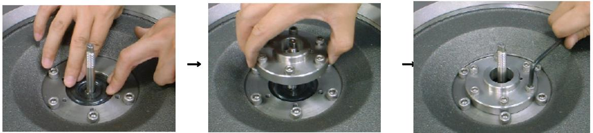
○Assembling the balance diaphragm
