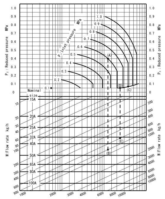
[Ex.1] For example, take a pressure reducing valve whose inlet pressure (P<sub>1</sub>) is 0.6 MPa, reduced pressure (P<sub>2</sub>) is 0.4 MPa, flow rate 800 kg/h. First, find the point of intersection (A) of inlet pressure 0.6 MPa and reduced pressure 0.4 MPa. Vertically proceed from point (A) to come across the flow rate 800 kg/h, and regard this point as (B). Point (B) is between nominal sizes 40A and 50A. Select the larger nominal size 50A.
