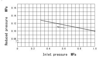
Reduced pressure is set to 0.1 MPa when inlet pressure is 1.0 MPa. The chart indicates a variation in reduced pressure when the inlet pressure is changed from 1.0 to 0.3 MPa.
