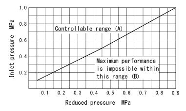
Find the intersection point of the inlet and reduced pressures. The GP-1200 (1210) valves are suitable within range (A). When within range (B), maximum performance cannot be obtained.
