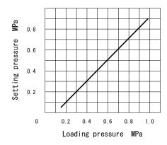
The setting pressures corresponding to the loading pressure are shown left. (P<sub>1</sub>: 1.0 MPa) As slight deviations from the loading pressure-setting pressure chart line shown left may occur depending on conditions, such as the length of the air line, etc., a setting pressure which is high enough to cover such deviations should be selected.
