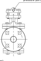
(mm) Size Н  $H_1$ Weight (kg) 150 220 15A 64 8.0 20A 155 220 64 8.5 67 235 25A 160 10.0 258 82 32A 190 14.0 14.5 190 258 82 40A 220 282 20.0 50A 93 65A 245 292 100 30.0 80A 290 339 122 35.0 330 100A 144 385 52.5
