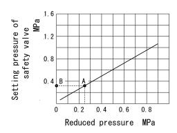
Determine the reduced pressure of pressure reducing valve. Find the intersection point (A) with the chart curve. Next, find point (B) by proceeds horizontally from point (A) to the left until the 'Setting pressure of safety valve' axis. The setting pressure of the safety valve should be higher than the pressure of the point (B).
