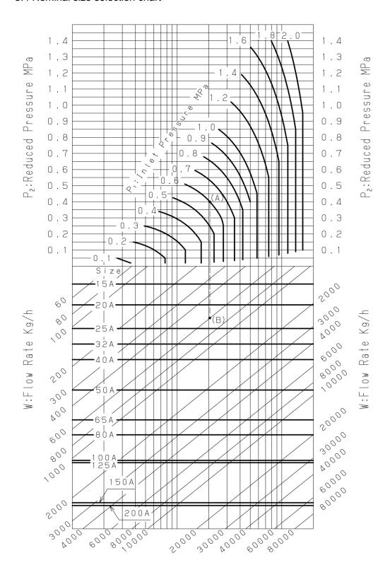
For example, take a pressure reducing valve whose inlet pressure (P<sub>1</sub>) is 0.6 MPa, reduced pressure (P<sub>2</sub>) 0.4 MPa, flow rate 600 kg/h. When determining the nominal size, find the point of intersection (A) of inlet pressure 0.6 MPa and reduced pressure 0.4 MPa. Vertically proceed from point (A) to come across the flow rate 600 kg/h, and regard this point as (B). Point (B) is between nominal sizes 20A and 25A. Select the larger nominal size (in this example, nominal size 25A)
