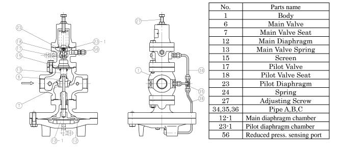
(1) When the pressure reducing valve is mounted correctly, releasing the compression of adjusting spring [24] allows main valve spring [13] and pilot valve spring [19] to close main valve [6] and pilot valve [17]. Slowly open the gate valve and allow the high pressure fluid to flow in. Inlet pressure is applied to the upside of the main valve. High pressure fluid passes through screen [15] to also apply inlet pressure to the downside of the pilot valve. (**Fig. 1**)
