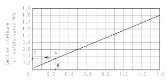
Reduced pressure of pressure reducing valve MPa
