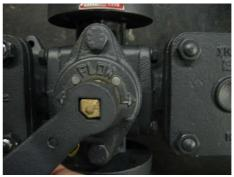
3. After switching, fit the adjusting screw to the hexagon hole on the handle and turn counterclockwise. When cock and adjusting screw turn at the same time, please fix the one side with the wrench. Please tighten the adjusting screw with provided handle.
