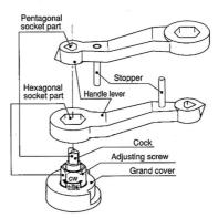
2. Fit the pentagon hole of the handle to the cock. (Stopper is facing downward) and switch the cock right or left. Match the arrows on the cock and handle with the arrow end on the screen side to be used. Turn until the handle stops by the stopper
