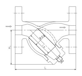
[Figure 1] 15-50A (No plug is provided with 15 to 32A ones.)
