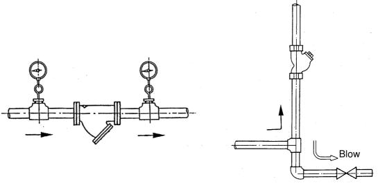
[Figure 5] Horizontal piping
