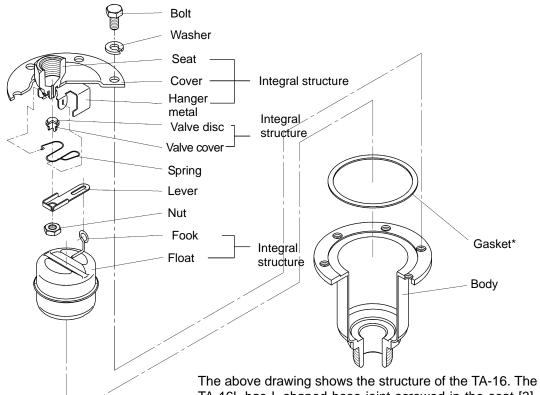
The above drawing shows the structure of the TA-16. The TA-16L has L-shaped hose joint screwed in the seat [3]. The TA-16CVA and TA-16CVS have check valve joints (the CV-16A and CV-16S respectively) screwed in each seat [3]. Parts marked with an asterisk (\*) are consumable parts.
