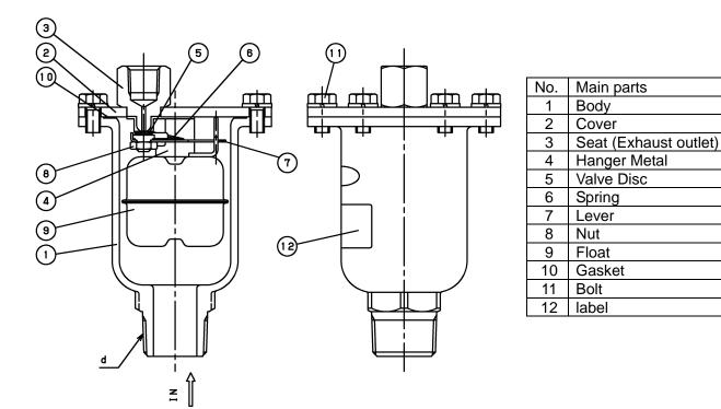
The above drawing shows the structure of the TA-16. The TA-16L has L-shaped hose joint screwed in the seat [3]. The TA-16CVA and TA-16CVS have check valve joints (the CV-16A and CV-16S respectively) screwed in each seat [3].
