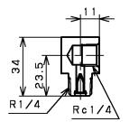
Check valve joint (angle type)
