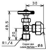
Manual valve with copper joint
