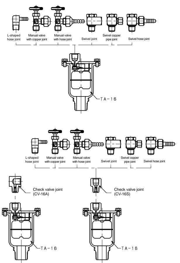
Caution: If check valve joint and swivel joint are used in combination, install the check valve joint to the TA-16 first, and then the swivel joint.
