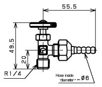
Manual valve with hose joint
