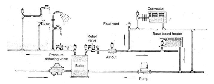
Using this product as a combination with Air Out (Air separator from water) type AO-2, it make efficiency of air discharge higher.
