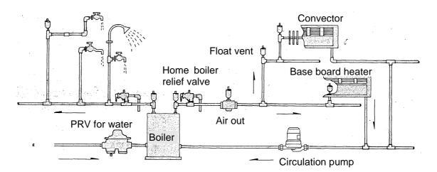
If using the product with AO-2 air out (air separator), higher performance can be obtained.
