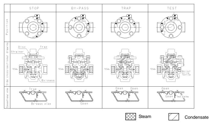
In order to switch the cock, be sure that each mark  $\blacktriangle$  of the functions meets the mark  $\blacktriangledown$  on the indicator accurately. If not, the product does not function correctly.
