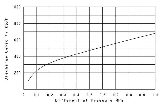
Max. continuous discharge capacity chart (Nominal size: 15A, 20A, 25A)
